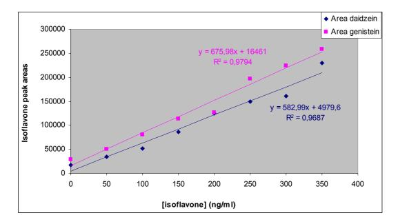
Fig. 19. Example of a calibration curve for determination of daidzein and genistein in rodent diet as a function of isoflavone peak areas vs. isoflavone concentrations (data from Table 16).
