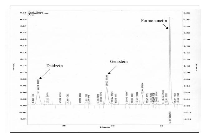
Fig. 18. Example of a chromatogram of a determination of daidzein and genistein in plasma (HPLC).
