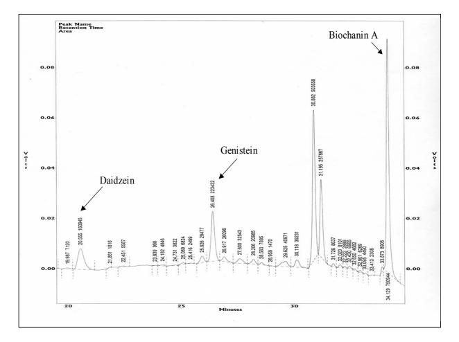
Fig. 17. Example of a chromatogram of a determination of daidzein and genistein in rodent diet (HPLC).
