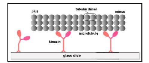
Fig. 14. Gliding assay: taxol-stabilised microtubules across a kinesin-coated glass surface (www.imb-jena.de).
