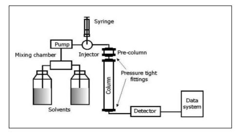
Fig. 7. Structure of a HPLC unit.
