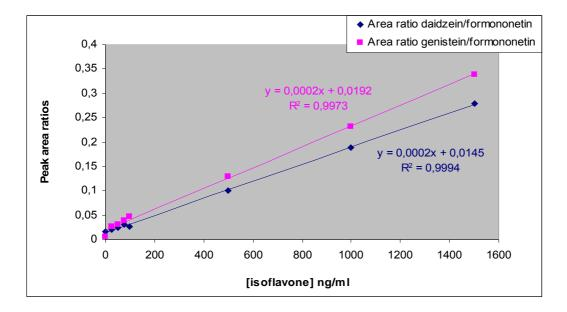
Fig. 22. Example of a calibration curve for determination of daidzein and genistein in rodent plasma as a function of peak area ratios vs. isoflavone concentrations (data from Table 17).
