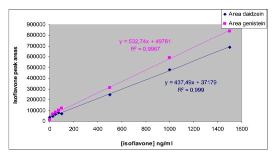
Fig. 21. Example of a calibration curve for determination of daidzein and genistein in rodent plasma as a function of isoflavone peak areas vs. isoflavone concentrations (data from Table 17).
