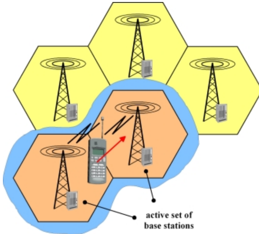
Figure 2.5. Soft-handover in 3G networks with an active set of two base stations
