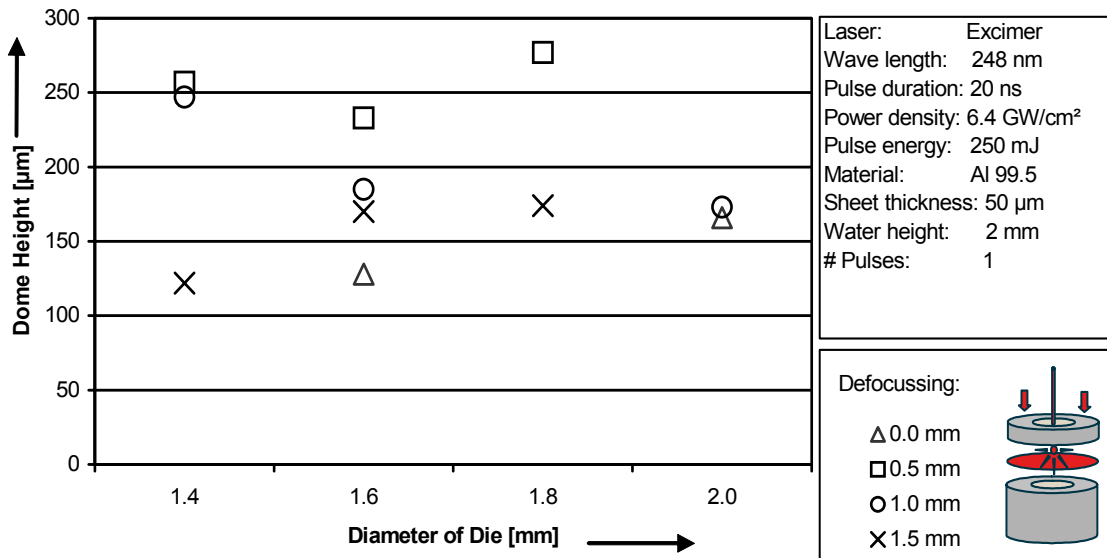
Figure 6: Dome height of laser stretch-formed parts depending on the defocussing (with use of a water film)
