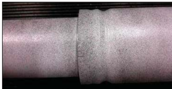
Figure 8: Detail of the test specimen with white layer and black speckle pattern
