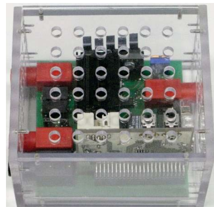
Figure 9. The complete HVDC-SSPC with the polycarbonate case
