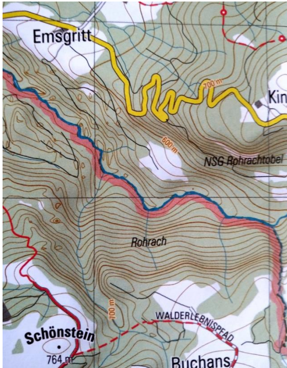
192 Scheidegg-Scheffau's hiking map uses contour lines in combination with hill shading and height points to give relief information. Contour lines with numbers are "index contours". (Scheidegg-Scheffau no date)
