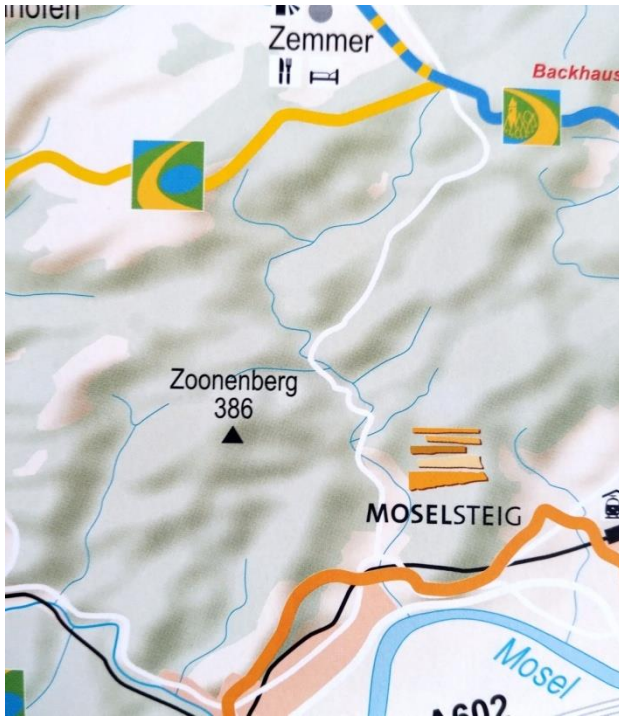
194 Hill-shading illustrates the relief in this map. Height points can be found on mountain peaks. Contour lines are missing. (Eifel 2016)
