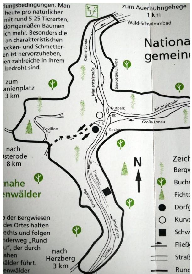
163 Although the map face offers enough free space for the labelling, the letters collide with other objects like the streets. Furthermore, the labels are not always placed where the named objects in reality are. (Harz 1995a)
