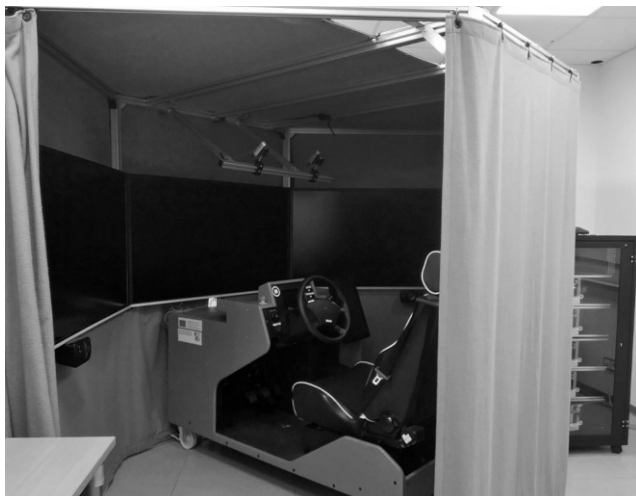
Fig. 6 Driving simulator of the Institute of Control Theory and Systems Engineering at TU Dortmund University. It was used for conducting the driving simulator study
