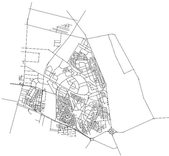
Figure 5.6.2. Drawn lines of roads of Andisheh new town in AutoCAD before importing it to the Depthmap software
