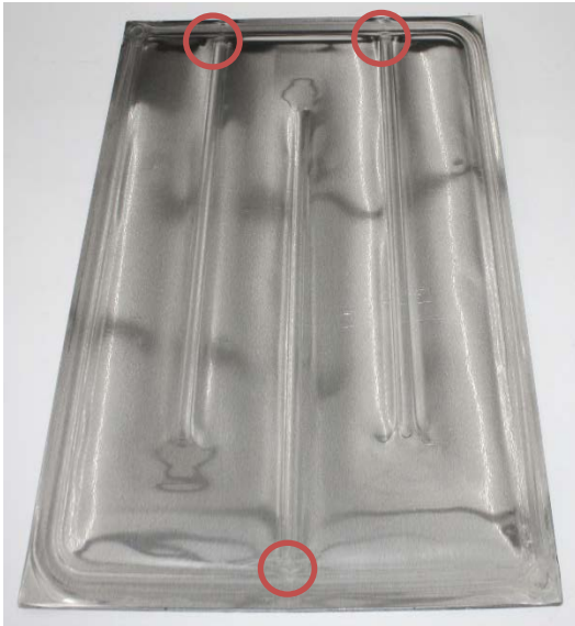
Figure 5: Cooling plate after welding
