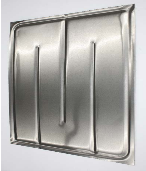
Figure 4: Preformed cooling plate before welding
