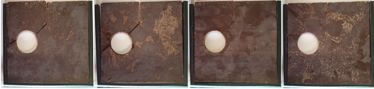
Figure 4.12: Cracking experiment of cooled dark chocolate: experimental specimens after cracking.
