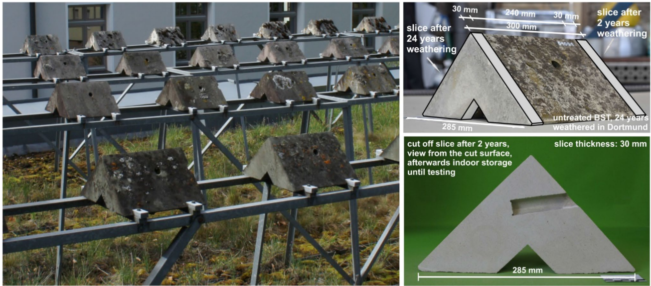
Fig. 1 Outdoor exposure field study and triangular prismatic shaped specimens of the Baumberger Sandstone, from which 30 mm thick slices were taken from the vertically oriented side surfaces after 2 and 17 resp. 24 years of outdoor weathering
