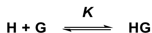
Scheme 3.2: Equilibrium reaction of host H with guest G to host-guest complex HG with binding constant K .
